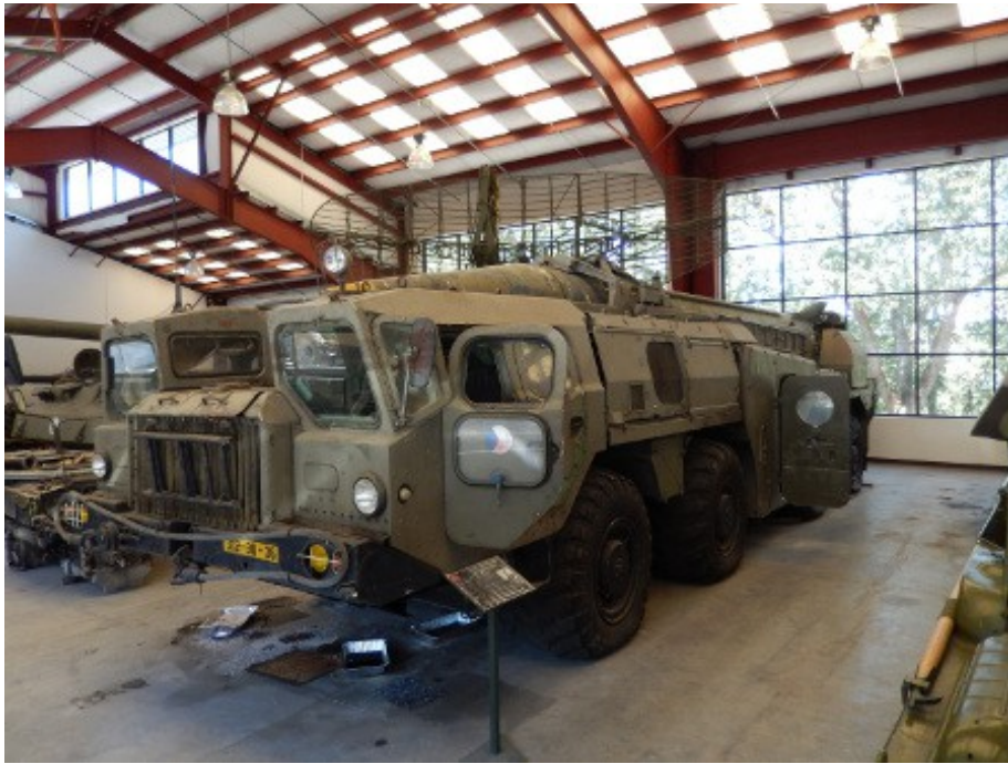
Top Left: A SCUD-B Missile Transporter/Erector/Launcher Bottom Left: The Long Track mobile SA-4 acquisition radar (30' long, 10.5' wide, 40 tons, 21 mph) Below: Some of the electronic assemblies inside the Long Track
