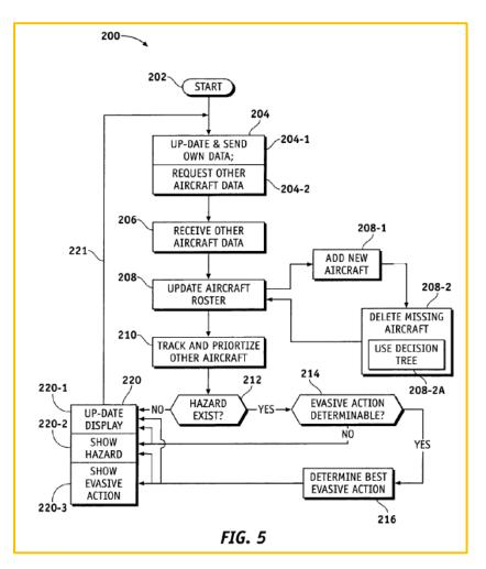
This patent is actually more comprehensive than ADSB traffic provides for – it's a Traffic Warning System which can give collision avoidance commands or advice. It's a little like TCAS, but thanks to specific data from other traffic giving their position, heading and altitude, we know range, time/distance and can make specific recommendations for traffic avoidance. Unfortunately, with the rapid development and adoption of WiFi, our patented box didn't go anywhere.
