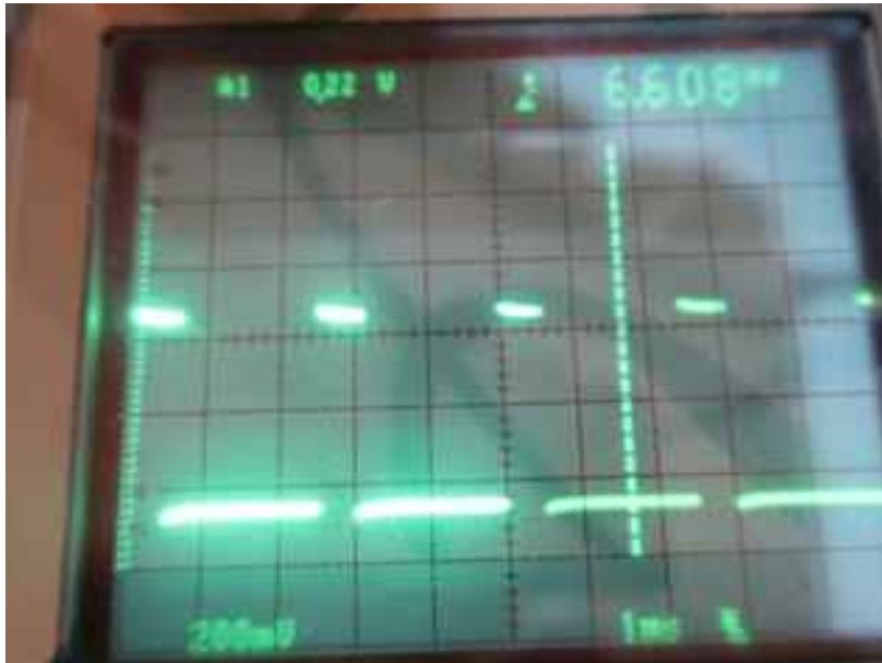
Figure 5 - NE555 .4/.1 sec gate signal
