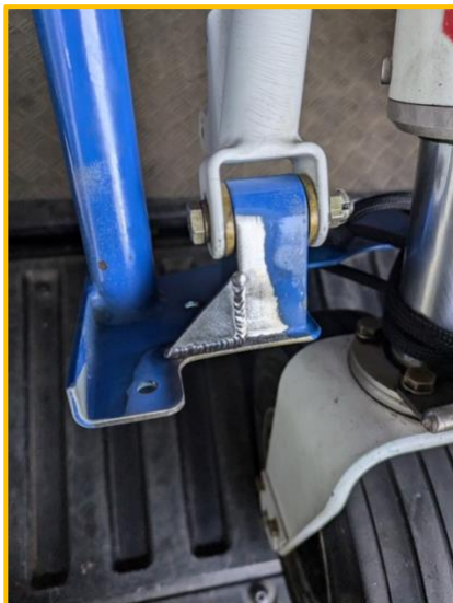
Completed weld with added gusset
