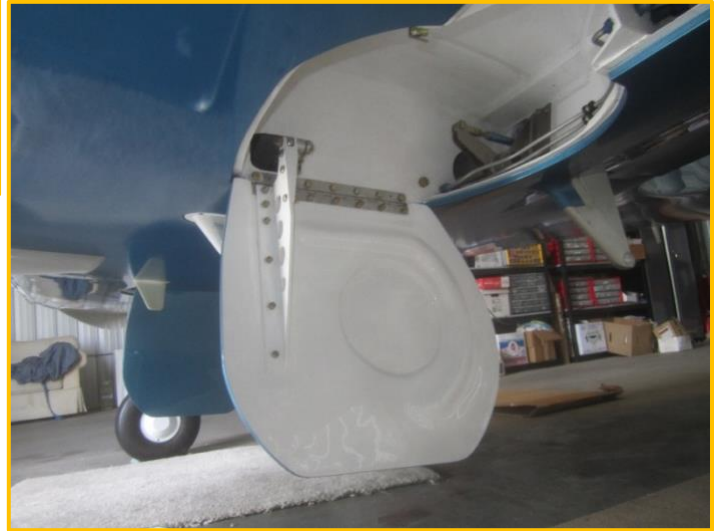
Correct hinges installed
