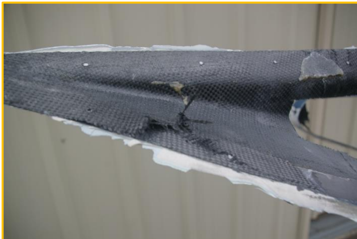
Infusion fillet with inadequate epoxy
