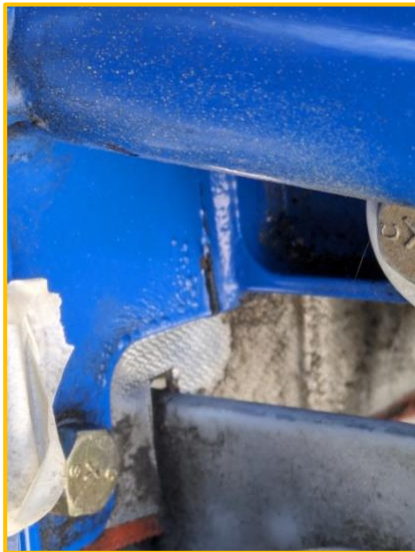
The dreaded engine mount crack (middle of picture)
