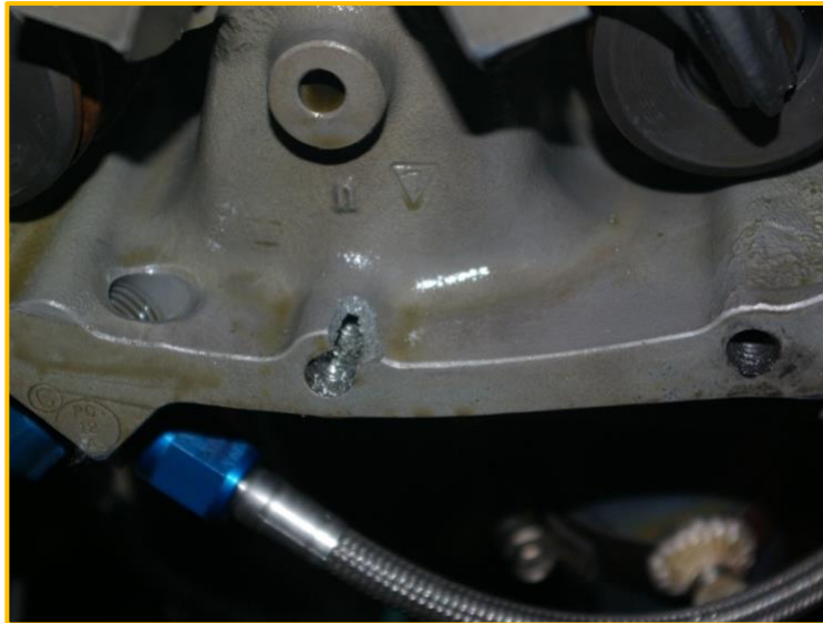
Damaged threads needed cylinder head welding (attach point for intercooler)
