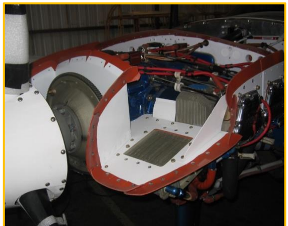
Final installation – flush with the intake panel and no exit restriction
