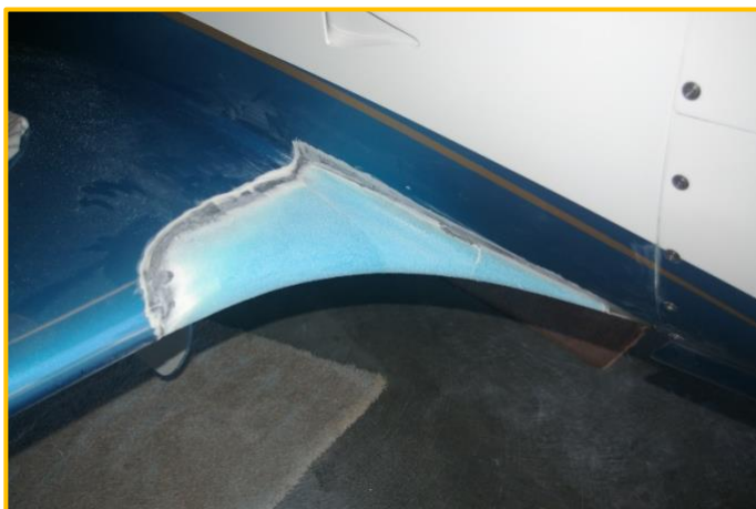
Old fillet removed, foam fillet form ready for covering
