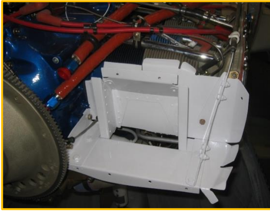
Initial Oil Cooler installation – blast air with vent to lower plenum
