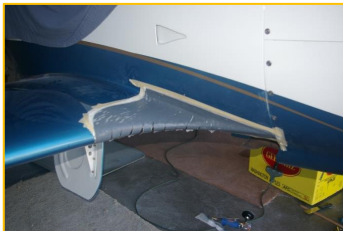
Replacement carbon fiber ready for finishing
