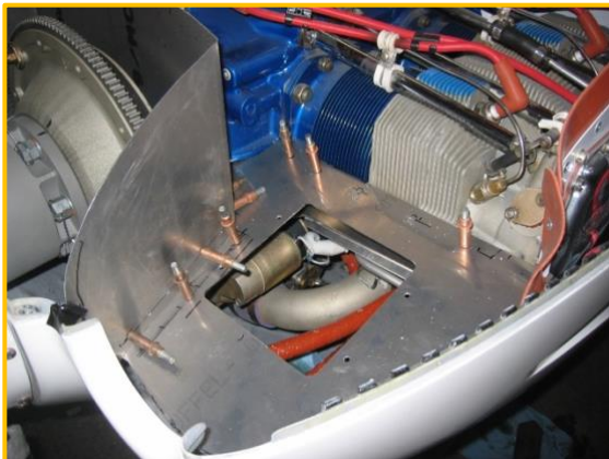
Rework installation – the way the factory did it
