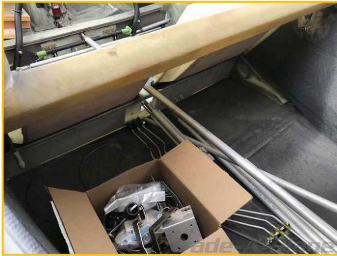
Hydraulic lines installed
