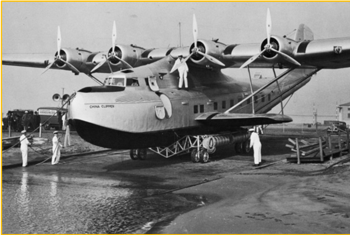
China Clipper on beaching gear (trolley) for freshwater wash and servicing
