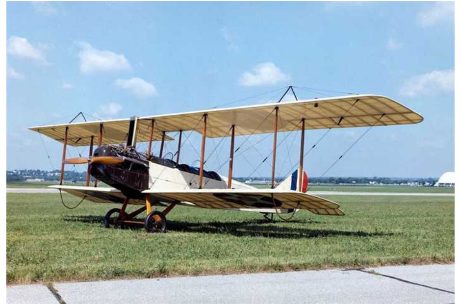
Curtis JN-4 "Jenny" to show a plethora of bracing wires
