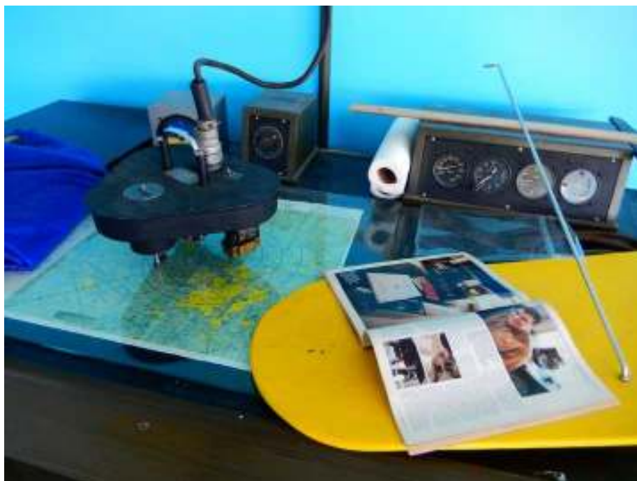
The Instructor's Station and plotting table. The vacuum tube electronics are in the desk drawer, below.
