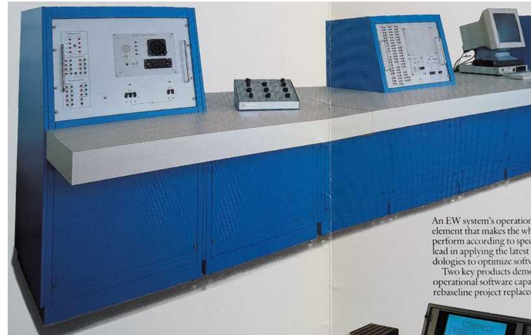
Test Bench built for the RAAF. The F/A-18's black boxes are mounted in the cabinets, cockpit indicators and test points on the front panels
